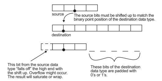
As the diagram shows, the source bits are shifted up so that the binary point matches the destination binary point position. The highest source bit does not fit, so overflow might occur and the result can saturate or wrap. The empty bits at the low end of the destination data type are padded with either 0's or 1's:
