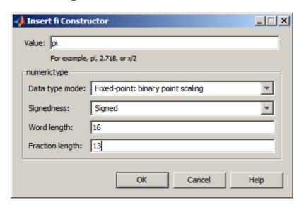
**3** To insert the fi object constructor string in your file, place your cursor at the desired location in the file, and click **OK** on the **Insert fi Constructor** dialog box. Clicking **OK** closes the **Insert fi Constructor** dialog box and automatically populates the fi object constructor string in your file:
