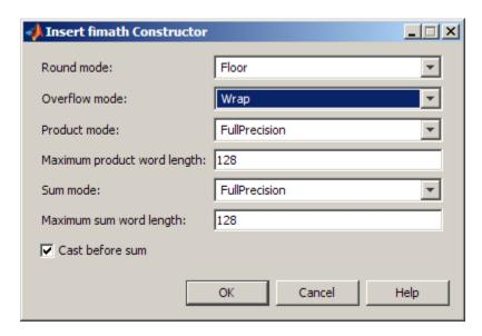
3 To insert the fimath object constructor string in your file, place your cursor at the desired location in the file. Then click **OK** on the **Insert fimath Constructor** dialog box. Clicking **OK** closes the **Insert fimath Constructor** dialog box and automatically populates the fimath object constructor string in your file:
